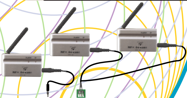
Front view of the RFX-150 with it's integrated RF LED. The RF LED offers installers a quick guide to an interference free mounting location.
